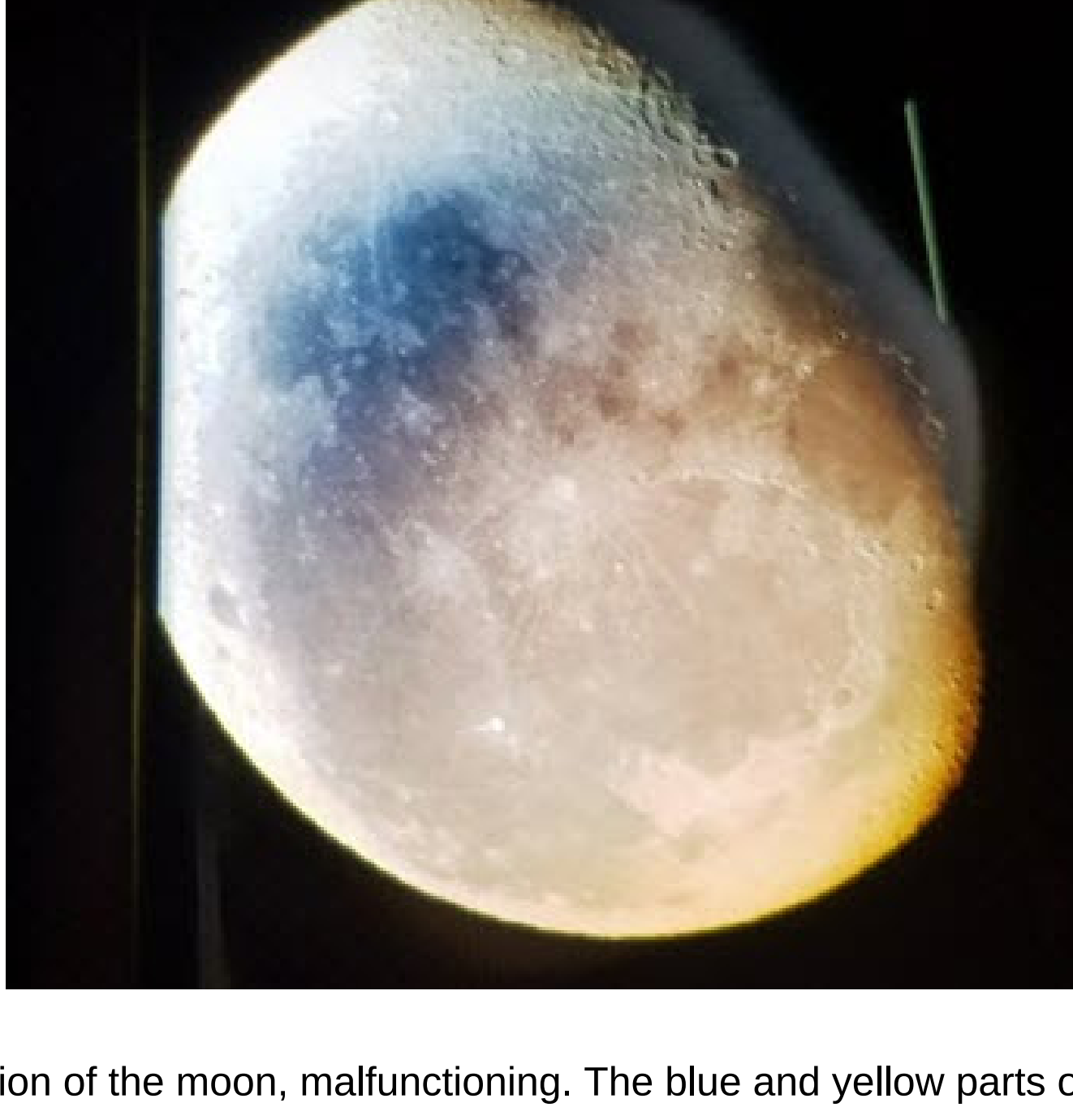
Figure 3. Holographic simulation of the moon, malfunctioning. The blue and yellow parts of the projection do not coincide and the image has completely broken apart on the top right (Source: Andrew from the Boogie Man channel).
