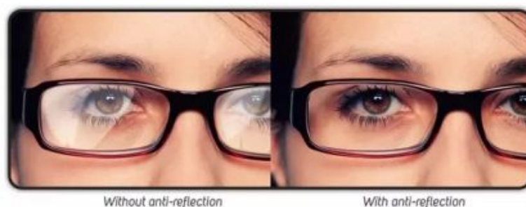
Figure 8.4. Thin films are used as anti-reflection coatings on glasses. They cause destructive interference of light reflecting off the lens so that it does not reach the eye.
